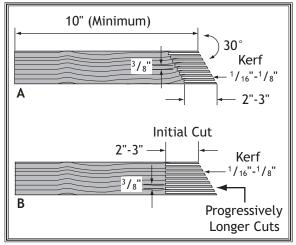
**Figure 63.** Patterns for making featherboards.
